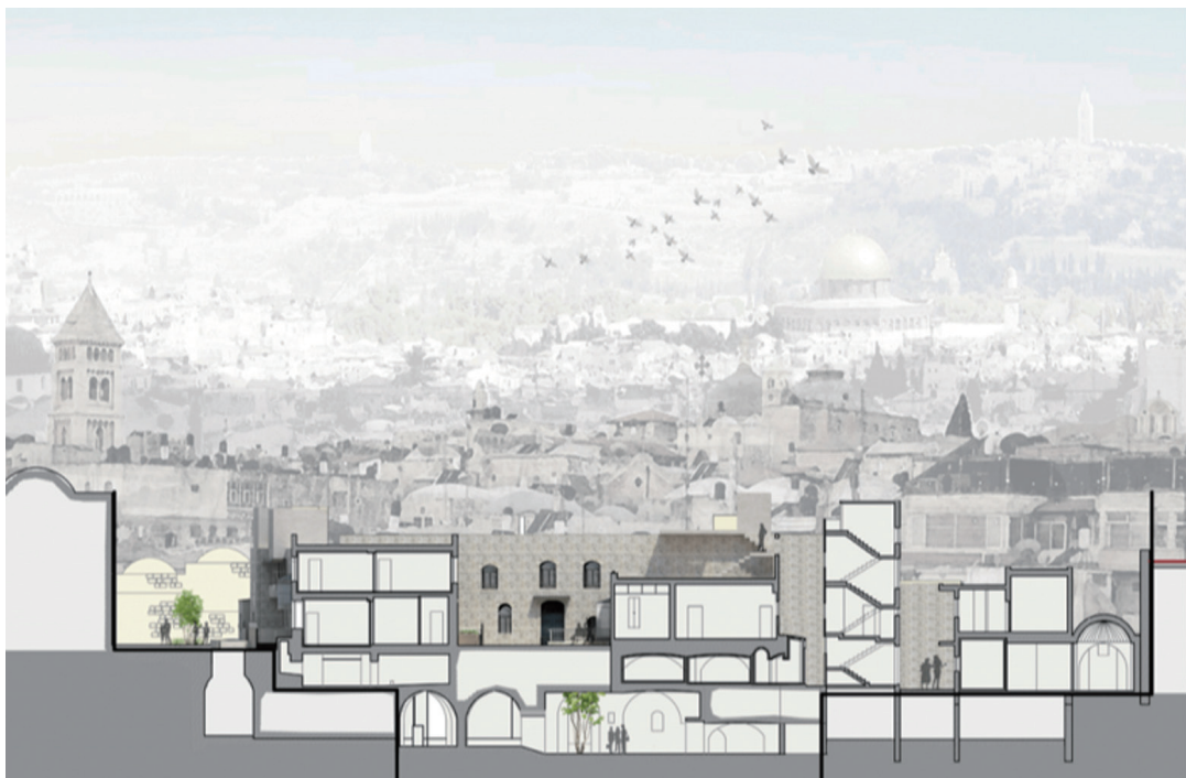
Figure 5.11 A sectional view of the complex that showcases the layering of multiple functions, the community and civic centre, residential units and open spaces
