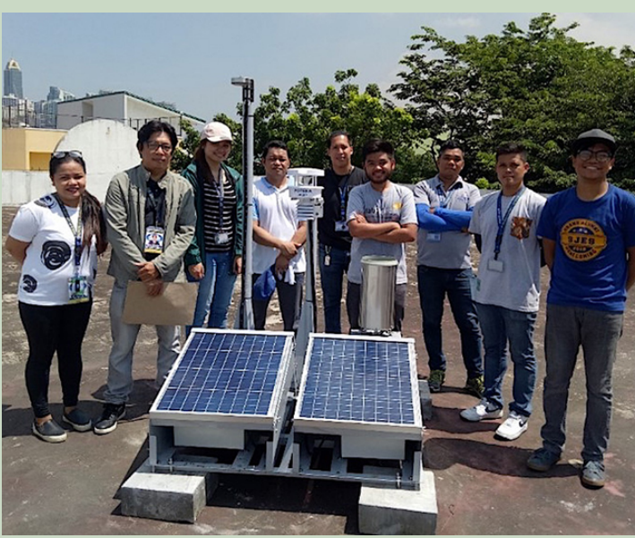
In 2021, DOST-PAGASA installed 40 lightning detection and automated weather stations all over Metro Manila and in selected regional Observation and Weather Stations. The system will provide data to determine the relationship of lightning strikes and torrential rainfall to put together a forecast method to predict the weather at a shorter time period
